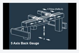
The TruBend 3000's 5-axis backgauge precisely positions blanks, guaranteeing accurate positioning of the panel and ensuring exact side length.
